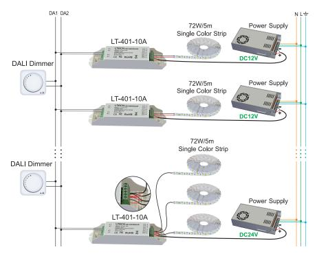
2) Providing DALI to 0-10V connect port, which is compatible to control 0-10V products in DALI control system, diagram example as below:
