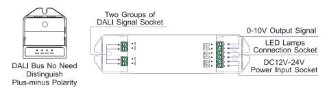
1) 12V lamp connected, loads 1~120W(12V), 24V lamp connected, loads 1~240W(24V),
